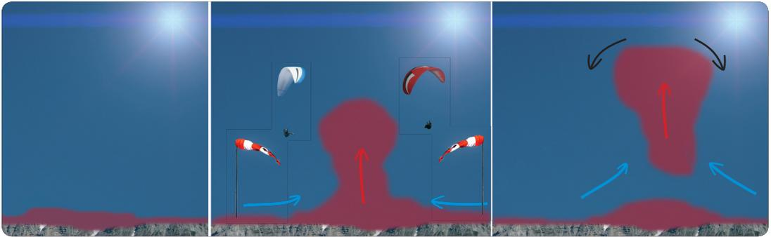
**Picture 1.3 A thermal is formed:** The ground is heated up by the sun and transfers some of the heat to the overlying air. At some stage the temperature difference becomes so great that the binding with the earth no longer holds. The thermal lifts off. Both pilots in the centre photo are flying with a tailwind!
